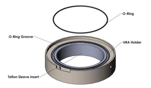
Figure 1. URA Holder with Teflon Sleeve Insert
