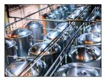
Fermentation and storage vessels (same as used in Agriculture) CO2 storage and filling machines (high & medium pressure disks, any suitable type)
