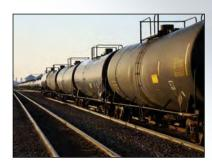
Generally graphite and metal rupture disks are used on a variety of applications. These include over the road intermodal tankers and railcar tankers. A variety of materials are available for these applications.
