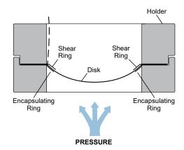
The process pressure is applied to the convex side of the RLP Disk placing the dome of the disk into compression. As the pressure rises past 90%, the dome becomes unstable eventually collapsing onto a shear ring that efficiently cuts the disk wide open upon reversal. The state-of-the-art shear ring allows the disk to function on both low pressure and liquid applications.
