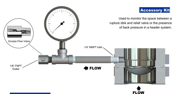
For proper use, excess flow valve should always be oriented either parallel to Earth or angled in an upward direction. Valve should never be angled downward during operation.
