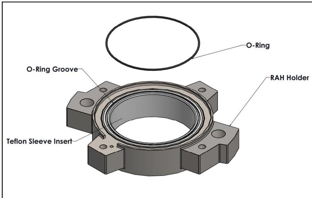
Figure 3. RAH Holder with Teflon Sleeve Insert
