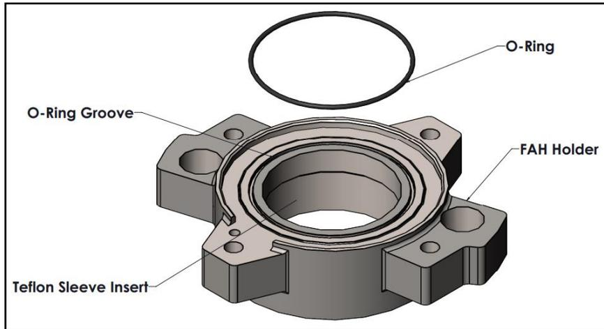
Figure 4 – FAH Holder with Teflon Sleeve Insert Cross Section
