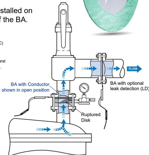
Relief Valve with BA & LD Burst Sensor Applications
